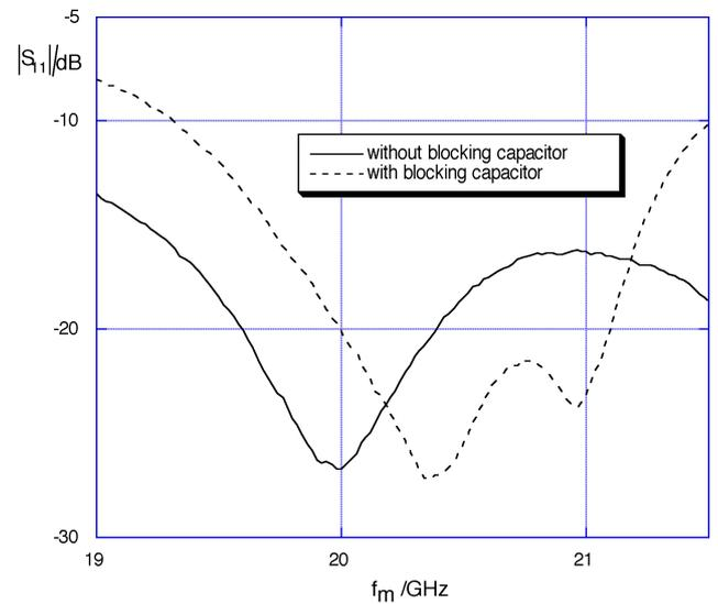
Fig 2: Modulus of input reflection coefficient  $|S_{11}|$  for single antenna element
