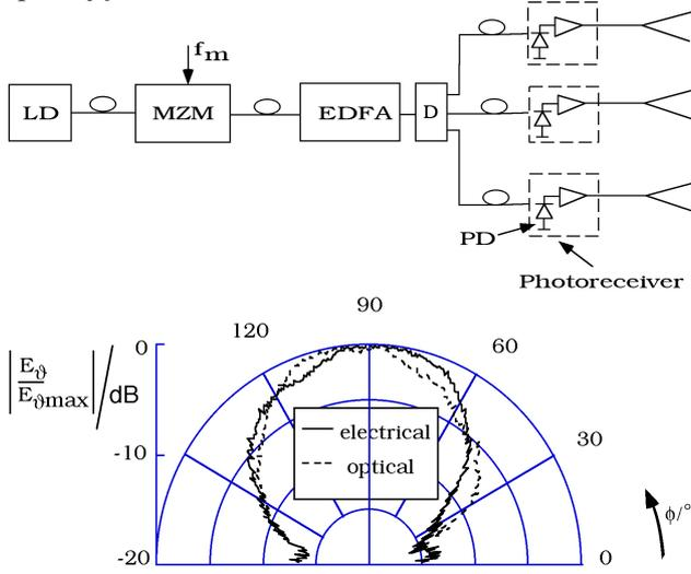
Fig 3: Measurement setup and H-plane radiation pattern of a single antenna element
