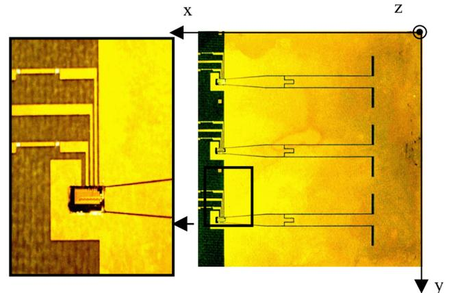
Fig 1: Antenna structure with embedded photoreceiver (PD) with a circular light-sensitive area of 10 μm diameter and a four-stage distributed amplifier made of pseudomorphic HEMTs. Each stage of the distributed amplifier consists of a cascaded pair of
