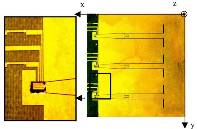
Fig 1: Antenna structure with embedded photoreceiver (PD) with a circular light-sensitive area of 10 μm diameter and a four-stage distributed amplifier made of pseudomorphic HEMTs. Each stage of the distributed amplifier consists of a cascaded pair of
