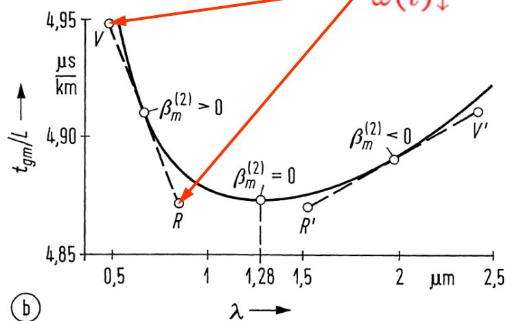
Intensity modulated monochromatic light source with chirp. (a) relative variance of received impulse as a function of the repeater length  $L$  normalized to the optimum value  $L_{op}$ . Chirp factors  $\alpha = 1, 2$ ; (o) chirp-free source ( $\alpha = 0, L_{op} = L_{op \max}$ ) (b) length-related group delay as a function of  $\lambda$  in a „waveguide“ mode (material dispersion for undoped quartz glass, Fig. 2.6)
