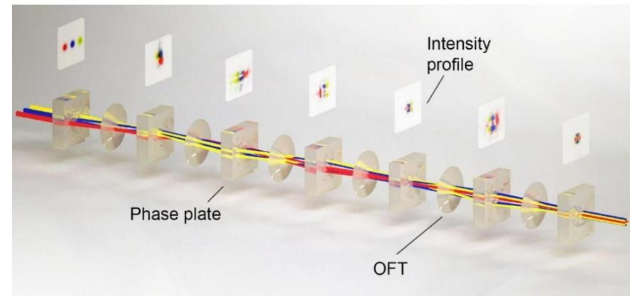
Multiple phase plates realize the transform of three adjacent Gaussian mode profiles into the desired fiber mode.
