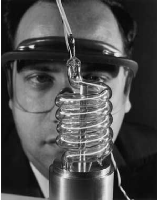
Theodor Maiman with the first ruby laser. (Photo: OSA)
