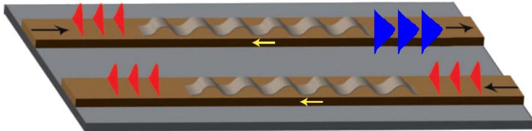
Illustration of how a travelling (dynamic) modulation of a silicon waveguide's refractive index can be used to perform optical isolation. The modulation induces a wavevector shift on light pulses (red) travelling from left to right, whereas pulses travelling right to left experience no such change. An optical polarization filter can be used to separate the shifted and non-shifted pulses.
