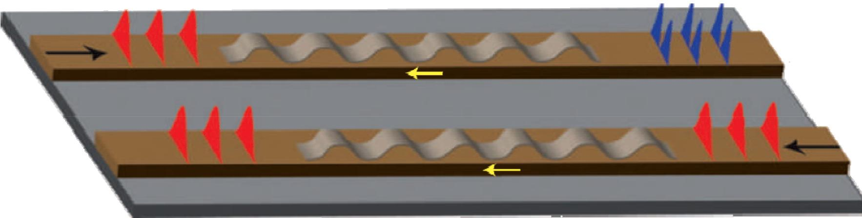
Illustration of how a travelling (dynamic) modulation of a silicon waveguide's refractive index can be used to perform optical isolation. The modulation induces a wavevector shift on light pulses (red) travelling from left to right, whereas pulses travelling right to left experience no such change. An optical filter can be used to separate the shifted and non-shifted pulses.
