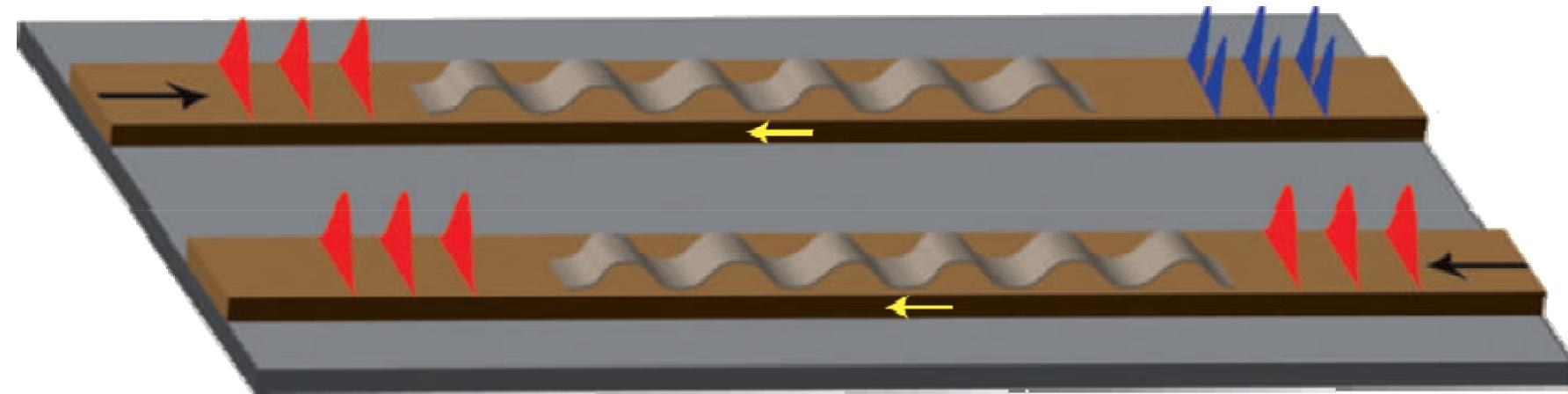
Illustration of how a travelling (dynamic) modulation of a silicon waveguide's refractive index can be used to perform optical isolation. The modulation induces a wavevector shift on light pulses (red) travelling from left to right, whereas pulses travelling right to left experience no such change. An optical filter can be used to separate the shifted and non-shifted pulses.
