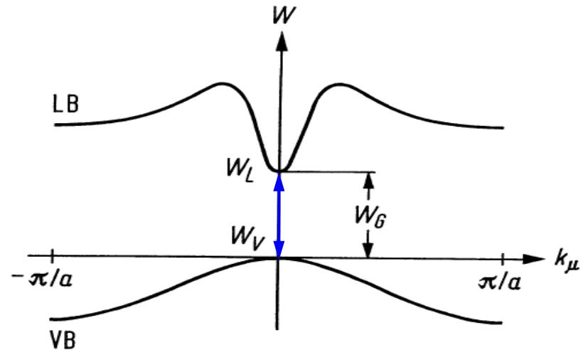
Indirect semicond. Smallest transition energy  $W_G$  for crystal momentum difference  $\Delta k_\mu = \pi/a$ . Phonon required for collision. Examples: Elemental semiconductors Si, Ge
