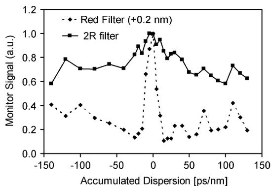
Fig. 5. Monitor signal for 40-Gb/s data as a function of accumulated dispersion.
