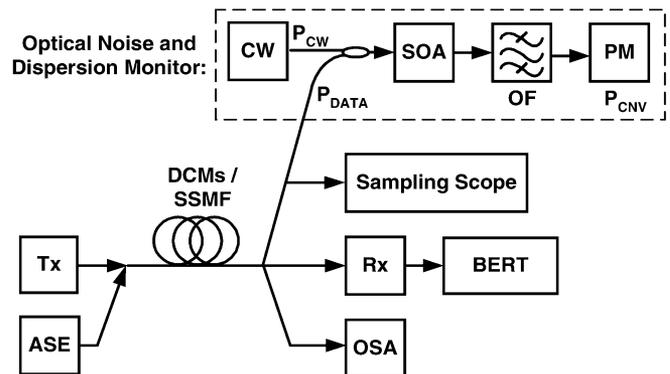
Fig. 1. Experimental setup to vary noise and accumulated dispersion on data signal  $P_{\text{DATA}}$ . The wavelength converted monitoring signal  $P_{\text{CNV}}$  is generated by mixing  $P_{\text{DATA}}$  with CW signal  $P_{\text{CW}}$  in the SOA and selected by the optical filter (OF). ASE: Amplified spontaneous emission source. CW: CW laser. Tx: Optical data source. PM: Power meter. Rx: receiver. BERT: Bit-error-rate tester.
