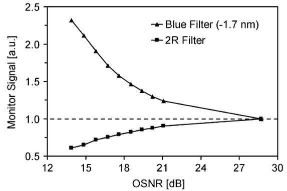
Fig. 3. Monitor signal OSNR dependence for two filter positions, normalized to the maximum OSNR value (40-Gb/s data signal).
