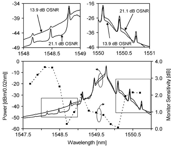
Fig. 2. SOA output spectrum at the converted signal wavelength and monitor sensitivity to OSNR changes. The two top figures are magnified views of the spectral regions that have the highest sensitivity shown boxed; 40-Gb/s RZ data signal was used.
