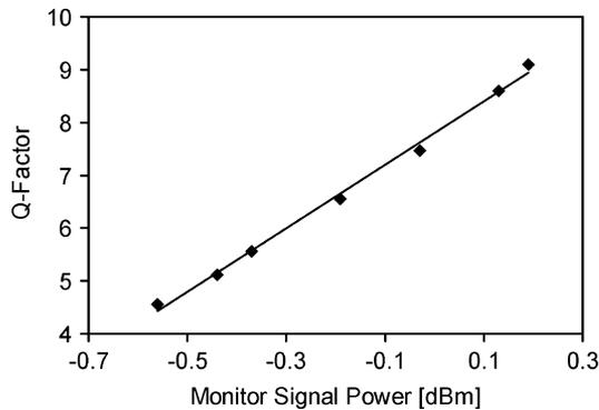
Fig. 4. Measured  $Q$  factor as a function of the monitor signal for the blue filter position when changing the OSNR (10-Gb/s data signal). The optical filter was in the blue position. A linear trend line is added for better visibility.
