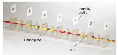
Multiple phase plates realize the transform of three adjacent Gaussian mode profiles into the desired fiber mode. Source: Labroille et al. Optical Fiber Technology 35. 2017.
