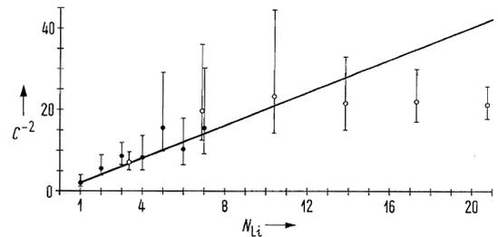
Fig. 1. Reciprocal squared speckle contrast in dependence of the number  $N_{Li}$  of independent patterns; —  $C^{-2} = 2N_{Li}$ , eq. (8); measured points:  $\circ$  fibre A,  $\bullet$  fibre B.
