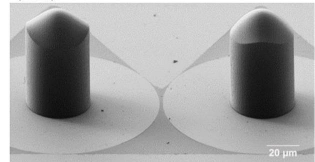
3D-printed lenses for coupling from an optical chip to a single-mode fiber (SMF). **a)** Lens on photonic-integrated circuit (PIC). **c)** Two anamorphic lenses on a SMF-array.
