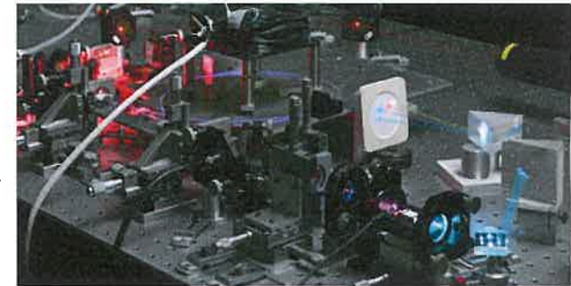
Fig.1: Demonstration laser setup including a \text{Tm}^{3+} -doped fiber laser
